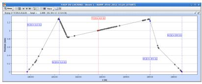
Inject with bump amplitudes of 0, 2 and 6 mm for TCDQ angles of 0 and ±1 mrad (possibly intermediate angles) around actual position → check loss pattern
