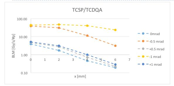
As expected higher losses for negative TCDQ angle. When the bump >2 mm → lower losses since TCDQ intercepts first the beam
