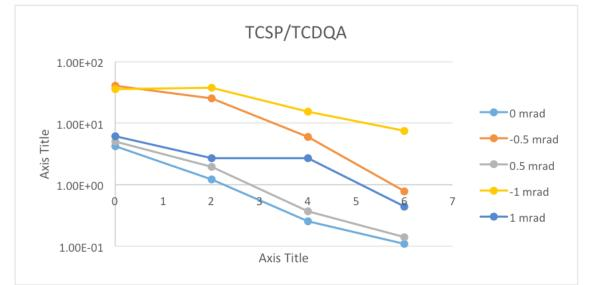
As expected higher losses for negative TCDQ angle. When the bump >2 mm → lower losses since TCDQ intercepts first the beam
