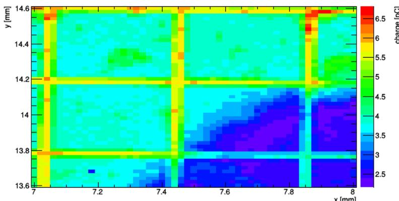
(TCT measurements on neutron and proton irradiated LGAD diodes.
