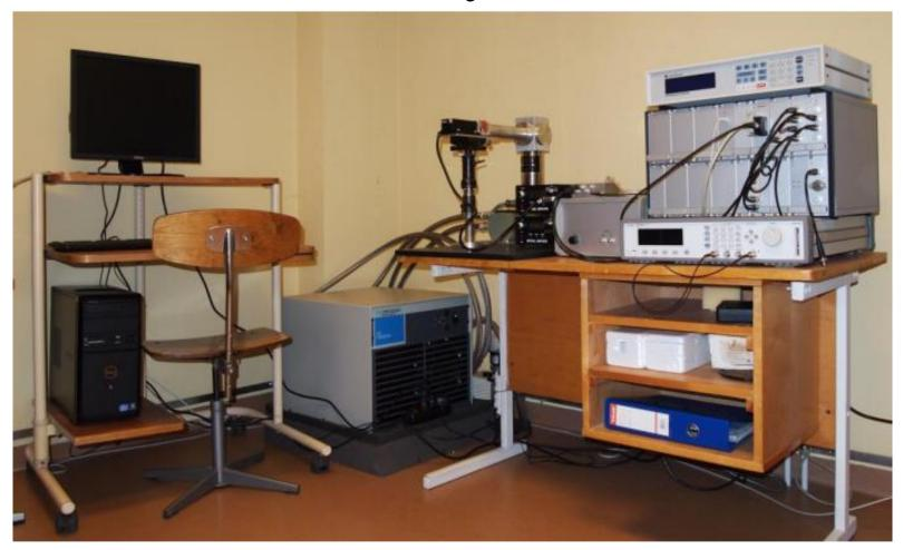
Hardware setup: PC, CTI-CRYOCRYOGENICS cryogenic system, CHAGCHUN NEW INDUSTRIES 1064 and 532 nm laser modules, Boonton 72B capacitance meter, Boonton bridge, LakeShore 336 Temperature Controller, Agilent 81107A pulse generator.
