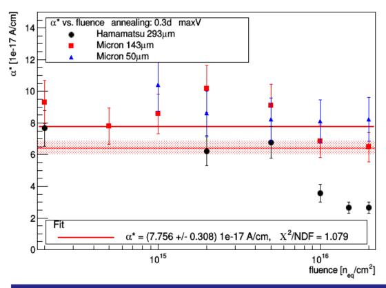
α\* shown for highest voltage (350 V for 50 μm-Micron, 1000 V otherwise)
