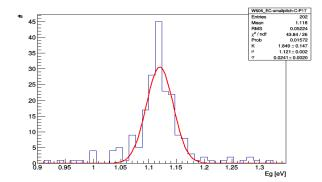
Measurement of unirradiated sensor results in expected value of  $E_{g,eff} = 1.12 \text{ eV}$ Ten IV-measurements of irradiated sensor at  $T = -23^{\circ}\text{C}$ :
