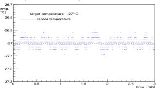
Measured sensor temperature does not deviate by more than 0.15°C from target temperature. (optimized PID parameters, unbiased sensor)
