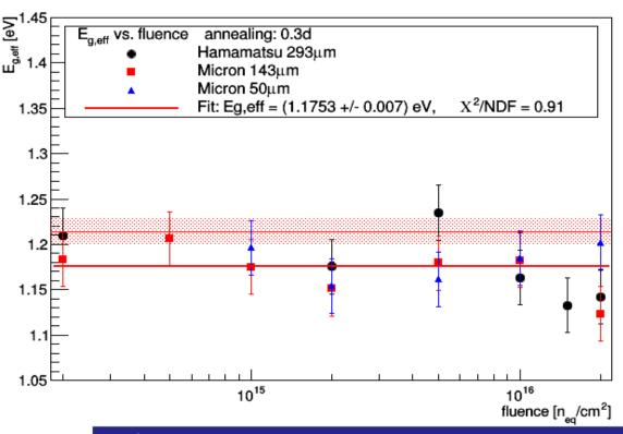
Additional measurement at -43°C and -39°C of 293um HPK-sensor,  $2x10^{16}$ neq/cm<sup>2:</sup>  $\rightarrow E_{a,eff} = 1.116 \text{ eV (-0.026 eV)}$
