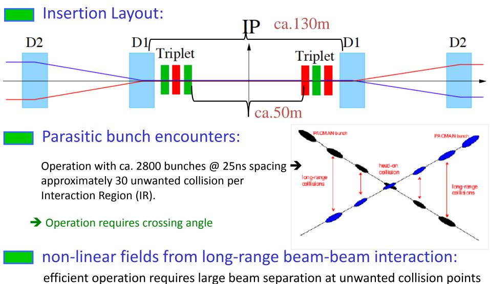
$\rightarrow$  Separation of 10 -12  $\sigma \rightarrow$  large triplet apertures & Luminosity loss!!
