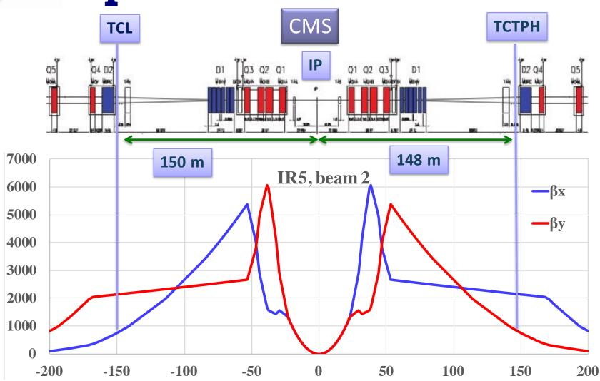
■ IR5: Horizontal TCT and TCL will be replaced with wire-embedded collimators
