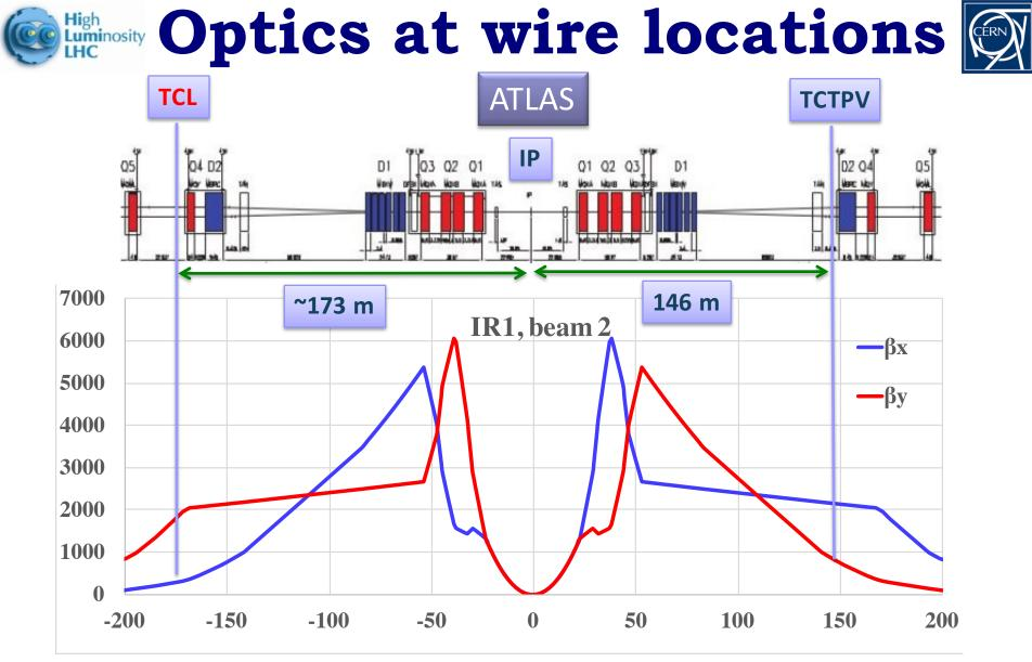
IR1: Vertical TCT will be replaced with wire-embedded collimator and **new TCL** installed downstream of Q4 (beam 2), as location next to D2 quite crowded
