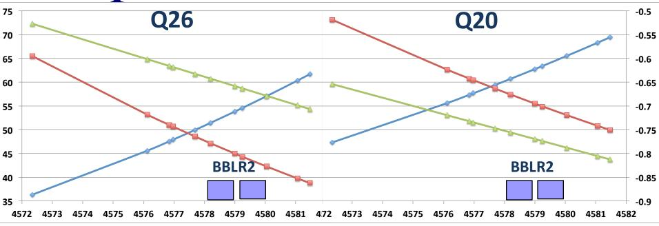
Q26 optics (nominal for FT beam)  $\square \beta_x \sim 53m, \beta_y \sim 45m, D_x \sim -$  0.65m  $\square Q20 optics (nominal for$ LHC beam)  $\square \beta_x \sim 63m, \beta_y \sim 55m, D_x \sim -$  0.75m
