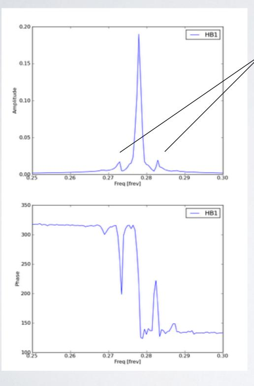
Synchrotron sidebands visible in the BTF signal
