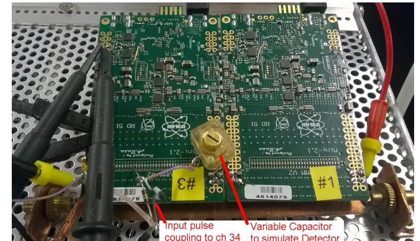
External pulse injection with variable "detector" capacitance
