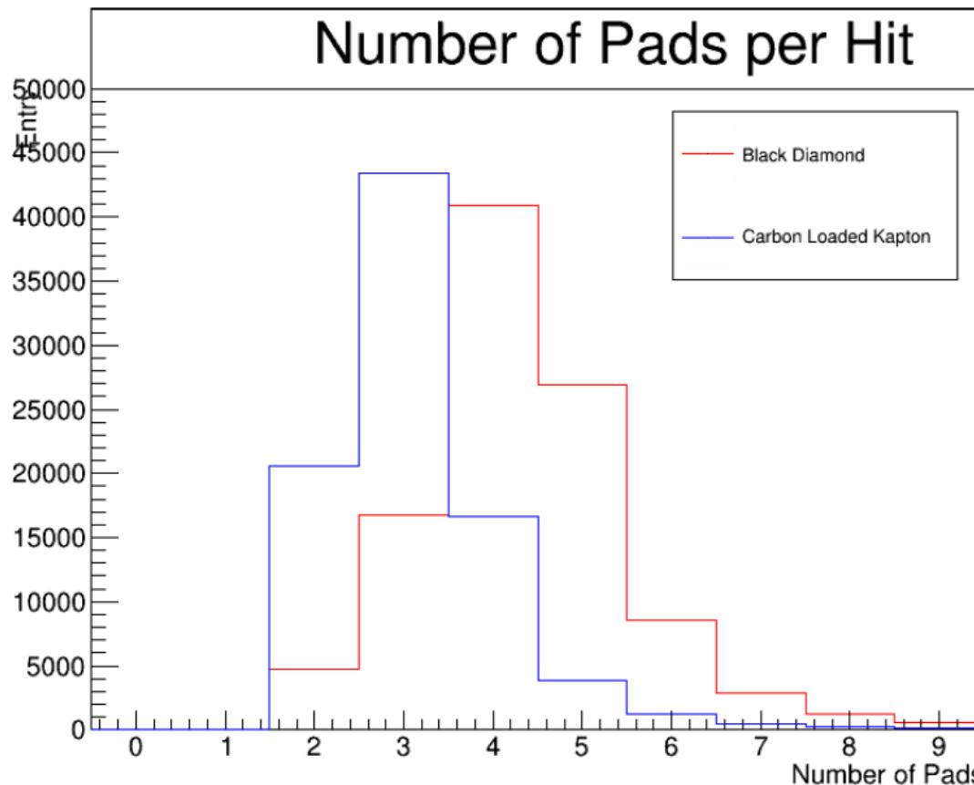
Number of pads that are fired when a charge cluster hits anode
