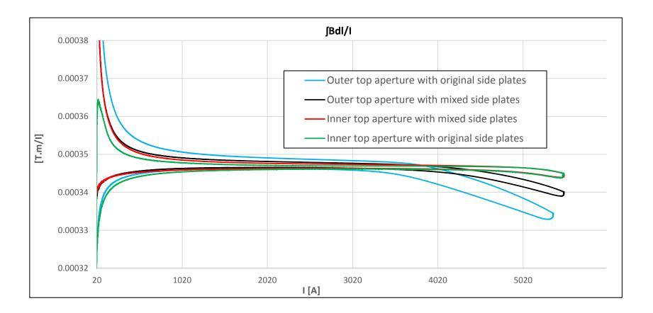
→ View of the saturation effects during a full current cycle, including eddy current losses (larger area inside the cycle)
