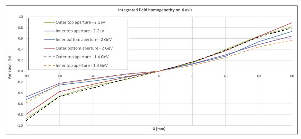
$\rightarrow$  Presence of a field gradient, but homogeneity better than  $\pm 1$  ‰ on  $\pm 80$  mm
