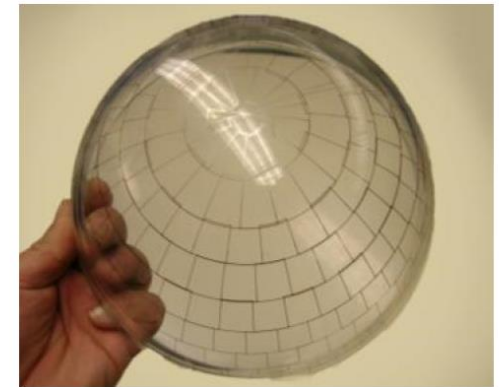
EMI Shielding Printed onto a Dome
