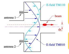
The **electrical center** is the point in which the electric field of the dipole mode (TMII0) is null and the picked up signal is at a minimum.
