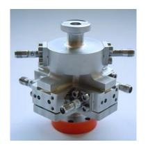
The CLIC RF-BPM has its dipole mode (TMII0) excited at ~I5GHz.
