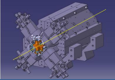
Two complementary interfaces, associated respectively to the geometrical center of the magnet and of the BPM
