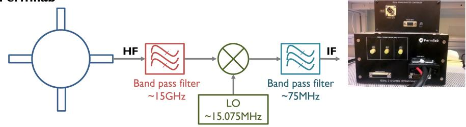
First tests with the 15GHz downconverter show resolution limits in the order of  $\sim$ 10um in the determination of the electrical center
