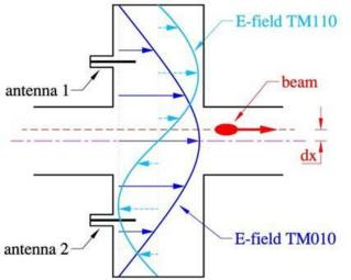
The signal is picked-up by **electrical coupling**, through four lateral antennas.
