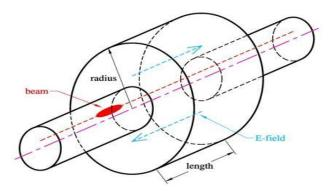
According to the spectrum of the beam, it couples with the monopole (TM010), dipole (TM110), and higher order modes
