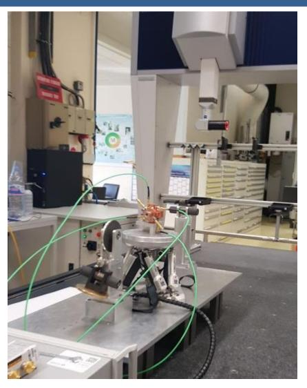
To accurately locate the position of the electrical center with respect to the wire the same measurements have been repeated in the metrology laboratory at CERN.
