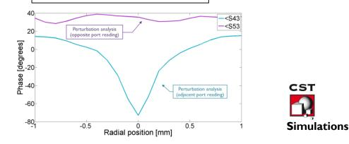
Scattering parameters (phase and magnitude), Sij: Excite from Port j and read from Port i
