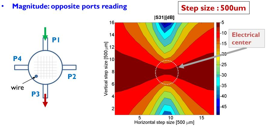
The wire behaves **as a probe** and couple the E-field in the cavity. On a larger scale we observe the **E-field pattern at the dipole-mode in two polarizations**
