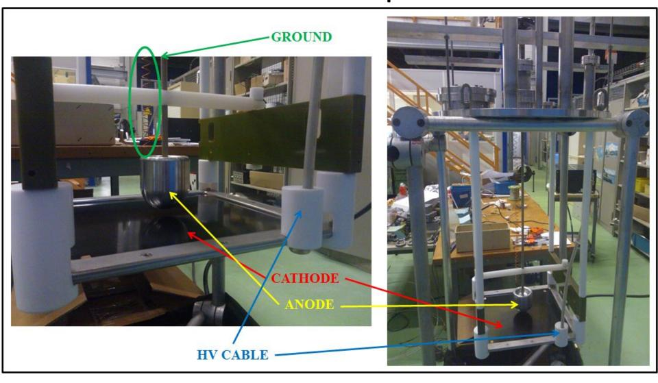
Resistive material is kept in position by SS frame. Connection with a small amount of silver paste. Sustaining structure for cathode plate and anode is in plastics (vetronite, teflon, PEEK).
