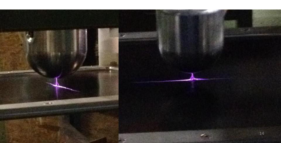
Status after test: degradation but no significant rip-off of material
