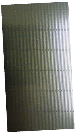
Rui also gave us a  $15x25 \text{ cm}^2$  sample of the Dupont resistive Kapton (3-4 M $\Omega$ \*cm bulk resistivity). Thickness is 25 µm, it need to be mounted on support for tests.
