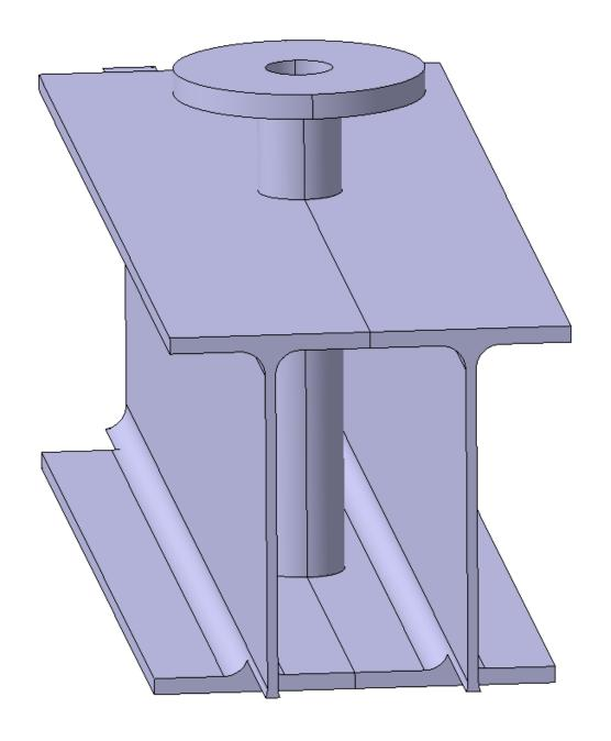
Supports for the feedthrus – Possible solution 1
