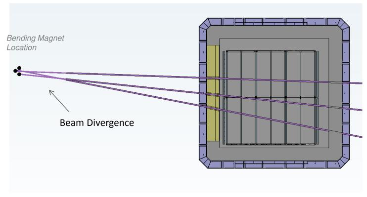
Second, set the ideal beam trajectories directly with respect to TPC elements. These beams may not trace back to the bending magnet, as can be seen by the divergence above.
