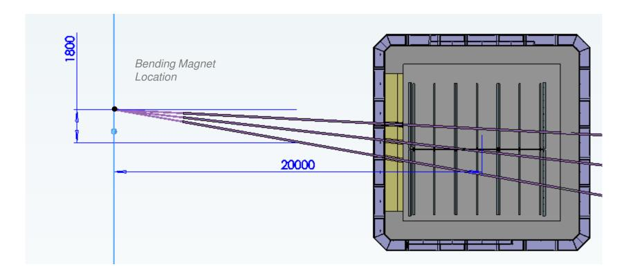
First, set the beamline elements, then determine where the beam can go. All beams diverge out from bending magnet, but may be constrained against ideal transit through TPC active volume.
