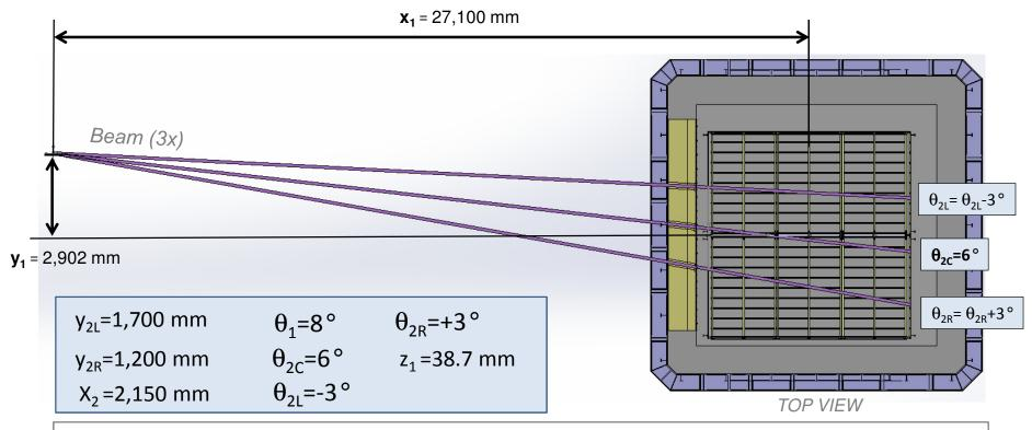
This is one possible set of eight values. These values are within range for the beam, plus the beams converge. However, the convergence point is approximately 12 m further than the initially proposed beamline layout, and this may not be feasible. Further values need testing.
