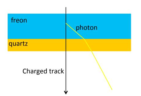
Mean freon refractive index is needed to handle, during the emission angle reconstruction procedure, the refraction of the Cherenkov photons at the freon/quartz interface.
