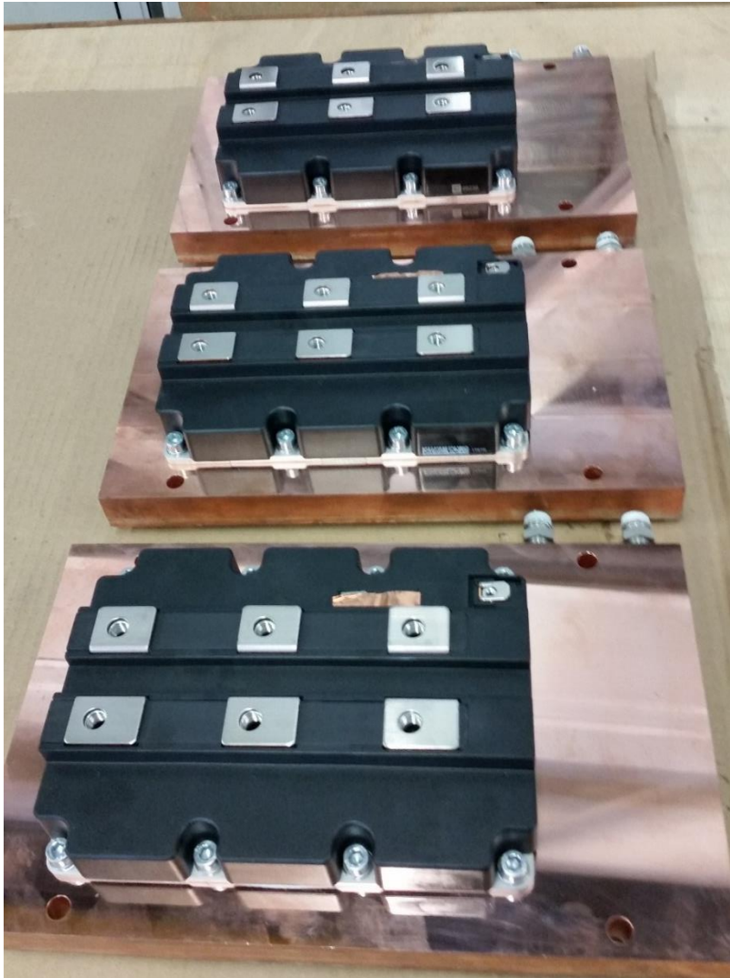
IGBTs on the heatsinks
