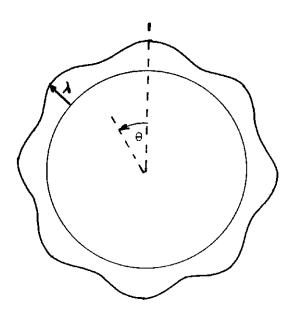
Typical perturbation Local line density of charge around a synchrotron
