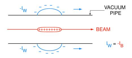
Wall current  $I_w$  due to circulating bunch Vacuum pipe not smooth,  $I_w$  sees an IMPEDANCE :
