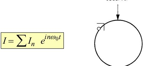
Produces a fundamental at the revolution frequency plus all higher harmonics are in equal strength
