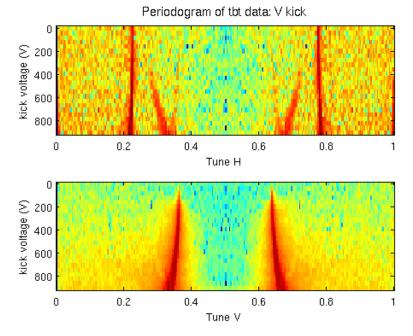
$Q_x$  seen in the V plane: (1,1) resonance  $2Q_x$  seen in the H plane: (3,0) resonance
