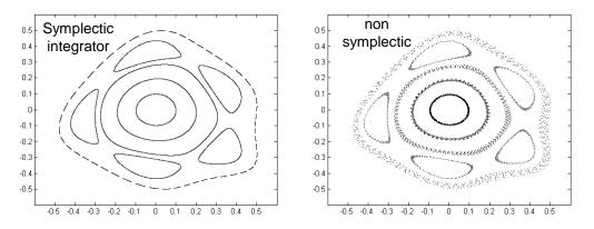
The well-known Runge-Kutta integrators are not symplectic. Likewise the truncated Taylor map is not symplectic. They are good for transfer line but they should not be used for circular machine in long term tracking analysis
