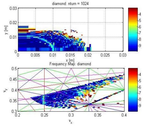
To each point in the (x, y) aperture there corresponds a point in the  $(Q_x, Q_y)$  plane
