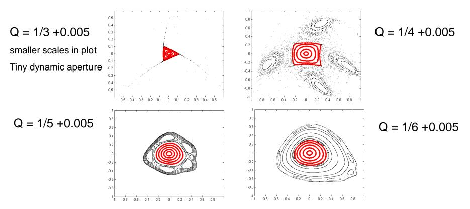
Tracking particles close to the resonant tune value, starting at the same tune distance from the resonance, show that a sextupole can excite all higher order resonances. The islands width is smaller for higher orders, i.e. the corresponding resonances are weaker
