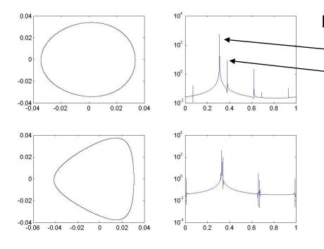
Far from the resonant values  $Q_x = p/3$  e.g.  $-Q_x = 0.31$   $-2Q_x = -0.62 \Rightarrow 0.38$ the lines  $Q_x$  and  $-2Q_x$  are well separated Approaching the resonant value  $Q_x = 1/3$   $Q_x = 0.33$   $-2Q_x = -0.66 \Rightarrow 0.34$ the tune spectral line ( $Q_x$ ) and the h<sub>3000</sub> spectral line (-2Qx) coalesce
