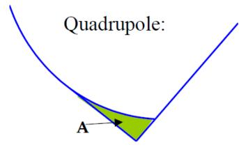
When high fields are present, chamfer angles must be small, and tapering of poles may be necessary
