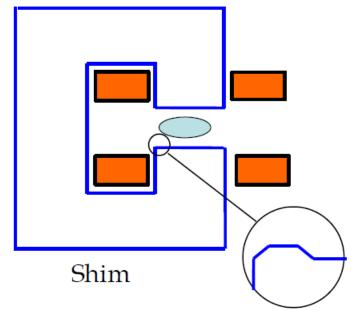
The 'shim' is a small, additional piece of fero-magnetic material added on each side of the two poles – it compensates for the finite cut-off of the pole, and is optimised to reduce the 6, 10, 14..... pole error harmonics.
