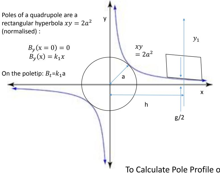
Combined function nagnet is like a quadrupole shifted by distance, h
