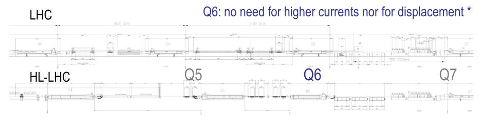
\*: ramp-down of Q6 is a limiting factor for Combined Ramp & Squeeze, enough room to be made available in RR in case Power Converters to be changed (1Q to 2Q)
