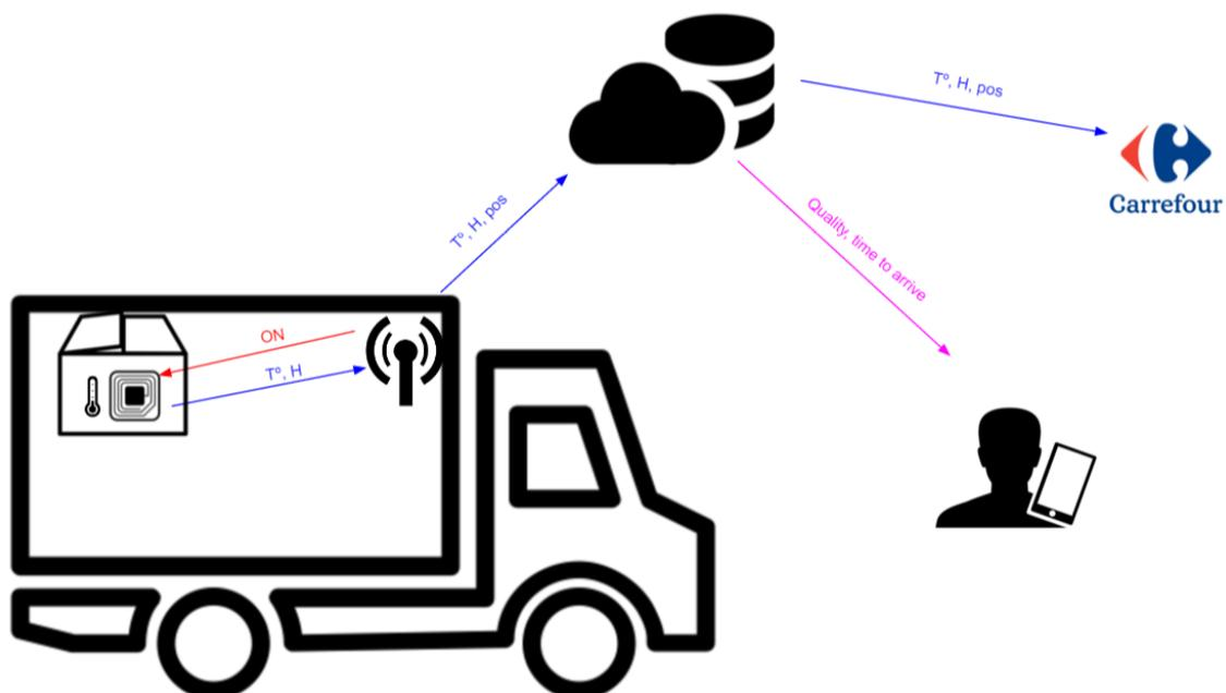
**Figure 7:** Tracking system final architecture
