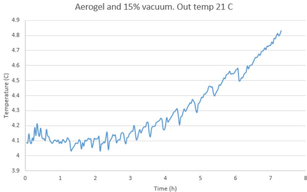
**Figure 5:** Aerogel test
