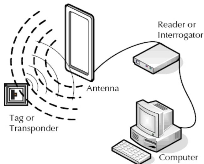
**Figure 6:** RFID simple architecture
