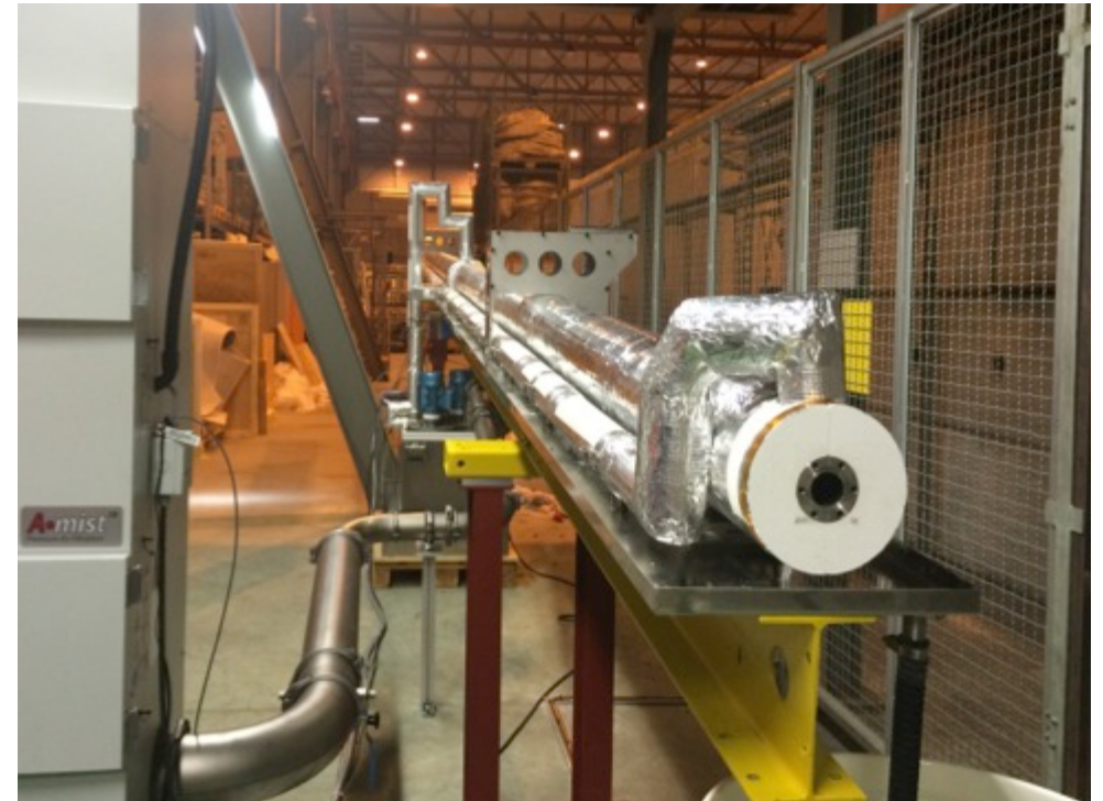
10 m long plasma cell prototype in the AWAKE test area at CERN
