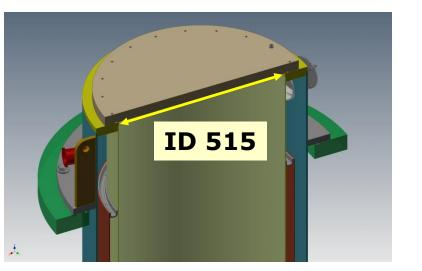
2.5 ton design load Conduction cooled thermal shield
