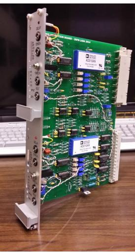
This old-fashioned, voltage-based, Quench Detection System to be integrated by other system(s) to be provided by the collaboration.
