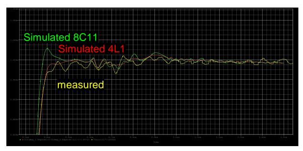
BT1.KFA10 Kick rise time (2-98)% -measured 121ns -simulated 8C11: 101ns -simulated 4L1: 125ns
