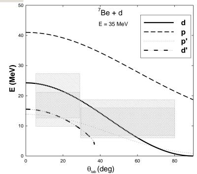
Kinematics of the 7Be(d,d), 7Be(d,p) reactions for ground state (d) (p), excitation of  $20 \, MeV(p')$ ,  $5 \, MeV(d')$  respectively. The forward hashed (backward hashed) areas cover the detected p (d) energies and angles in CD and barrel detectors of T-REX.
