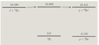
FIG. 1. Schematic illustration of the proposed  ${}^{7}\text{Be}$  destruction mechanism,  $d + {}^{7}\text{Be} \rightarrow {}^{9}\text{B}^* \rightarrow p + {}^{8}\text{Be}^*$ . The energies are in MeV relative to the ground state of  ${}^{9}\text{B}$ . Subsequently,  ${}^{8}\text{Be}^*$  breaks up into two  $\alpha$  particles.
