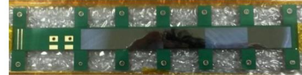
MFT Ladder prototype with fake sensors
