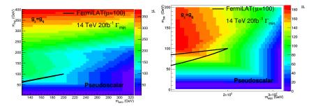
Plots illustrate the contours of the required  $\mu$ -factor necessary to enhance the signal for pseudo-scalar messenger models to set a 90% CL at 14 TeV LHC 2. The question of whether a parameter point is visible at the LHC depends on the ability to separate signal processes from the background. A better background rejection boosts sensitivity independently of the signal parameterisation and the real analysis sensitivity improves substantially:
