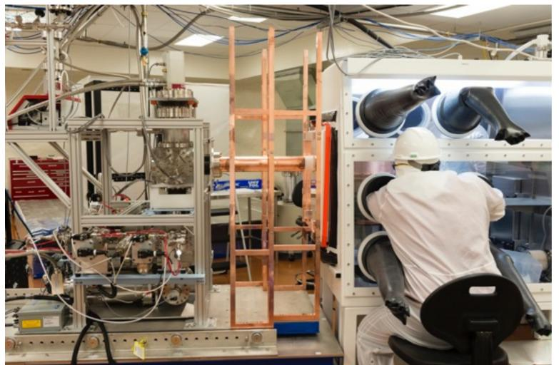
Prototype Cryostat with three installed strings
