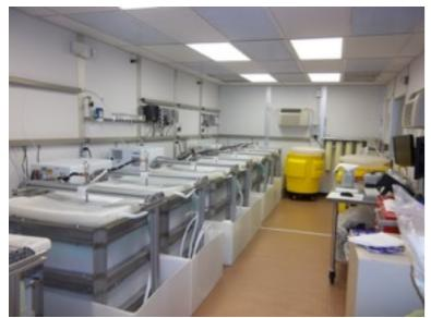
Electroforming Baths in TCR Inspection of EF copper on mandrels
