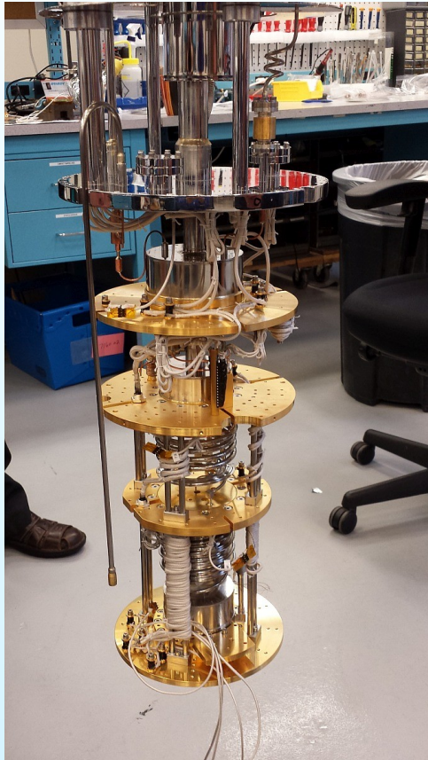
Dilution refrigerator under test. Currently being packed for shipment to UW.
