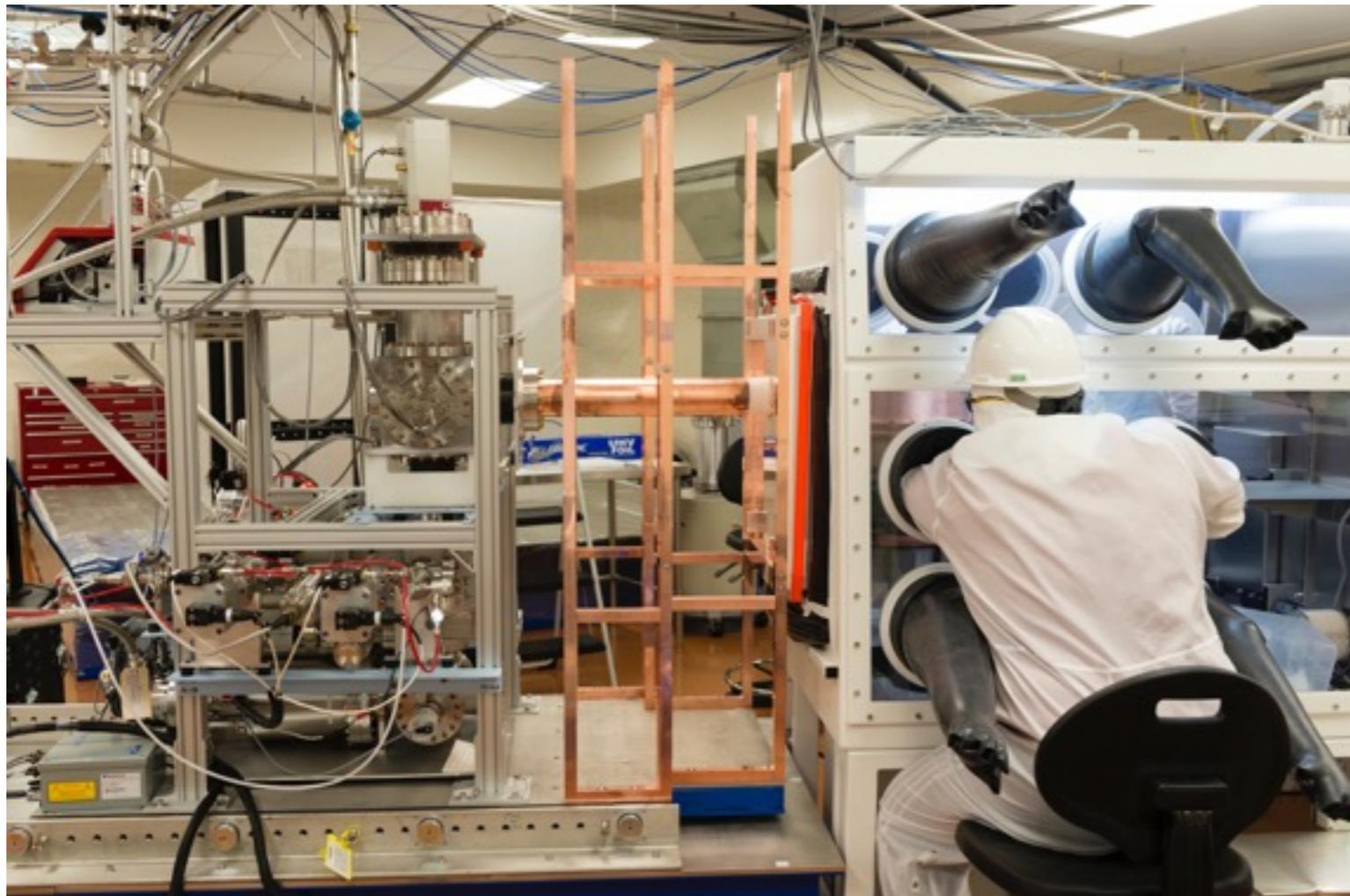
Prototype Cryostat with three installed strings
