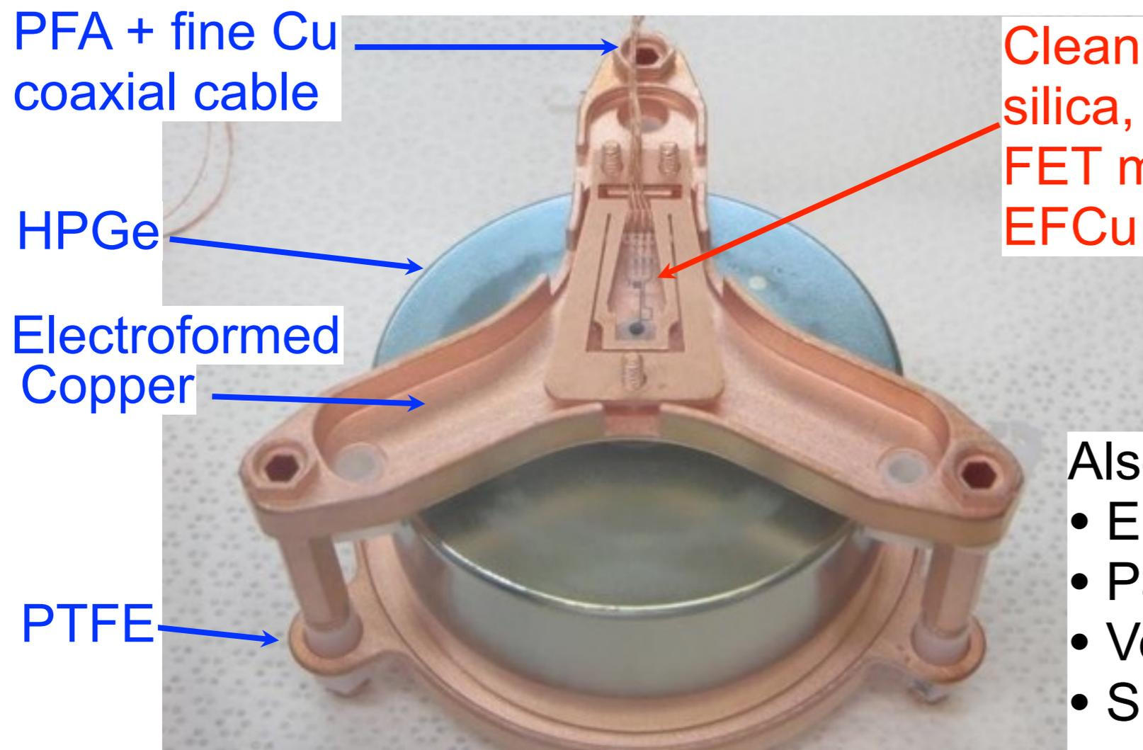
Clean Au+Ti traces on fused silica, amorphous Ge resistor, FET mounted with silver epoxy, EFCu + low-BG Sn contact pin
