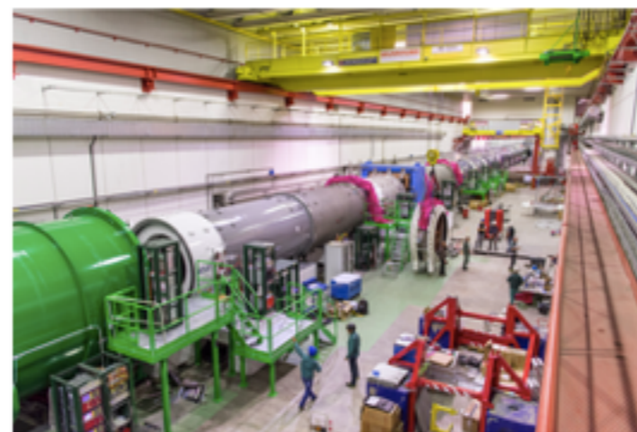
The 115 metre long vacuum tank of the NA62 experiment.
