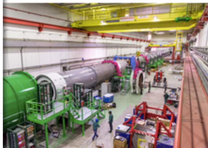
The 115 metre long vacuum tank of the NA62 experiment.
