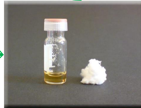
Solvation of cellulosic material in ionic liquid. The figure shows 5% (w/w) cellulose dissolved in [AMIM][Fo].
