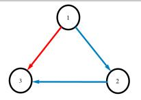
$$e_2 = e_1 + \rho \frac{v_{12}^2}{2}, \quad e_3 = e_2 + \rho \frac{v_{23}^2}{2} \quad \rightarrow \quad e_1 = e_3 + \rho \frac{v_{31}^2}{2}$$
