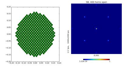
FWHM of the primary peak is 23.5 arcmin. Fraction of power on secondary peaks is around 70%
