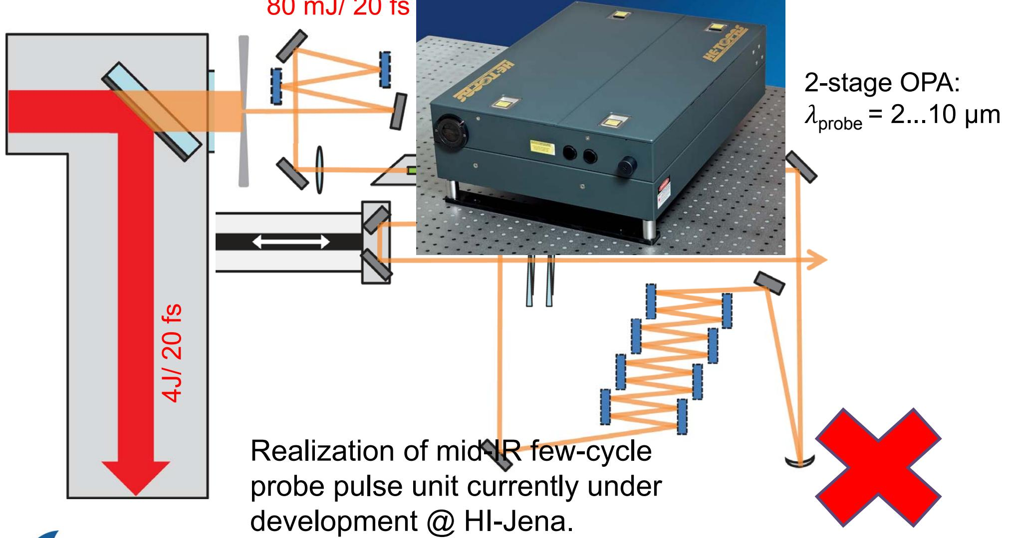
Synchronized probe pulses for laser-plasma interactions:
