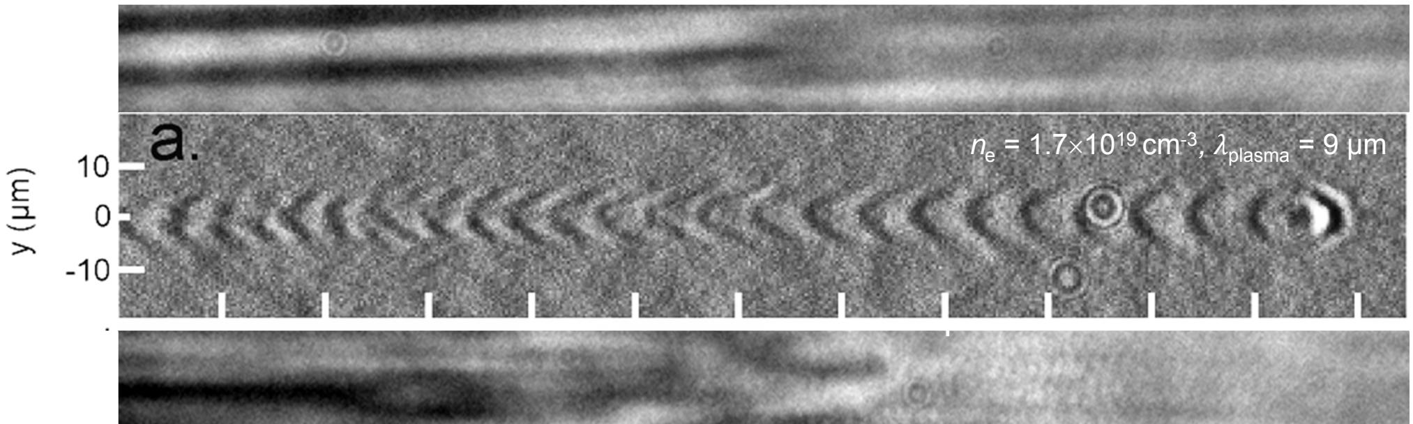
High-resolution ( $\mu\text{m}$  and fs) visualization of plasma wave and its evolution
