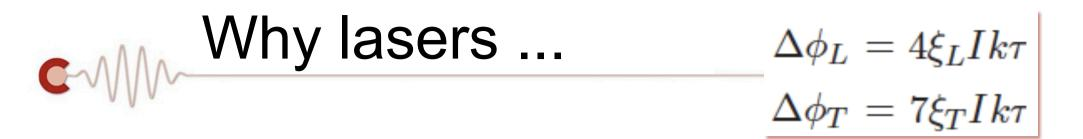
Photon-photon coupling results in a phase shift of the probe
