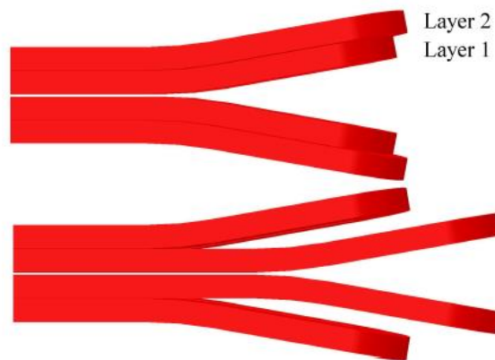
Figure 4: Coil design of HD2 (top) and configuration optimized to reduce integrated harmonics in the ends (bottom).
