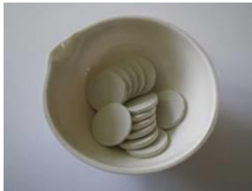
SiC pressed pellets (Saint-Gobain)
