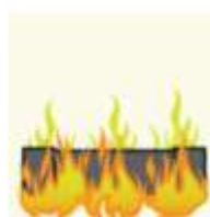
THERMAL A 30-minute, fully-engulfing fire at 800° (1475°)
