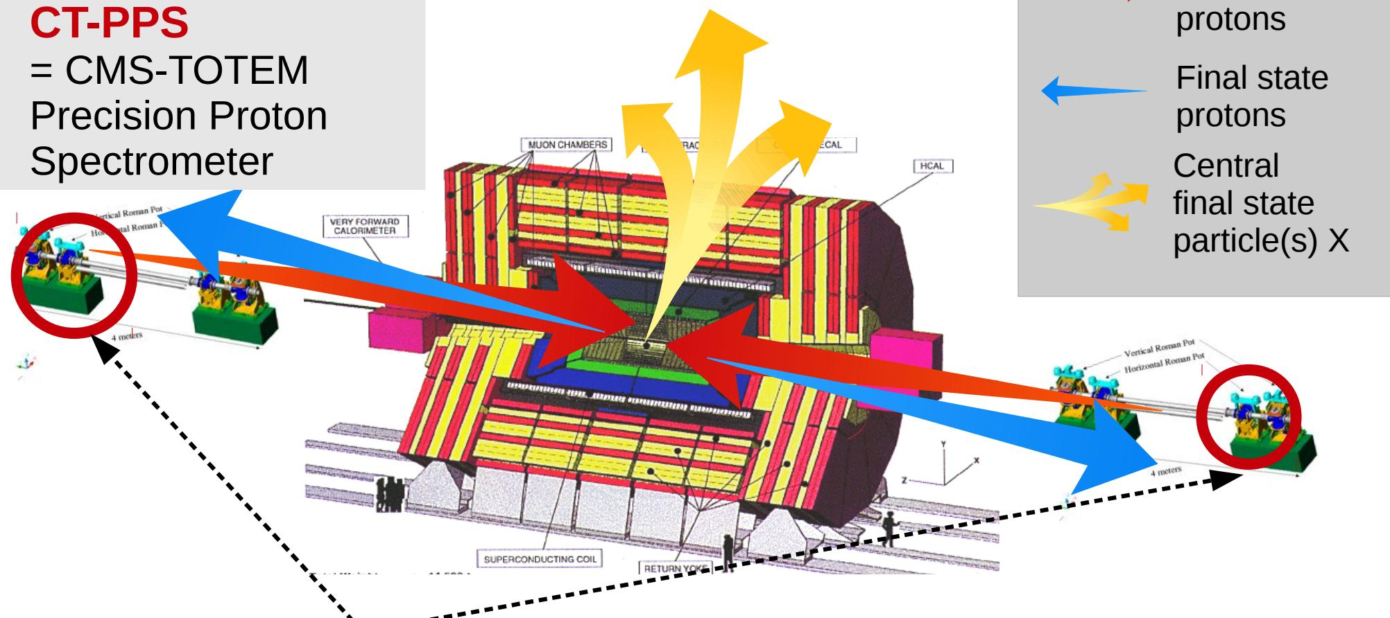
Time of Flight detectors  $\rightarrow t_1 - t_2 \sim z\text{-vertex}$
