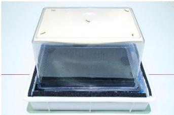
Place your plastic container upside down onto your metal plate. Fit the box so that the box walls fit the grooves in the metal plate. Now your chamber is ready to detect particles. It will only take a few minutes until everything has cooled down and a stable sensitive area has formed.
