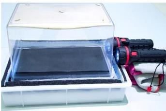
At first, you will only see a rain-like mist of alcohol. Place your torch lights in a way, that they illuminate the alcohol mist right above the metal plate – that is the sensitive area of the chamber.
