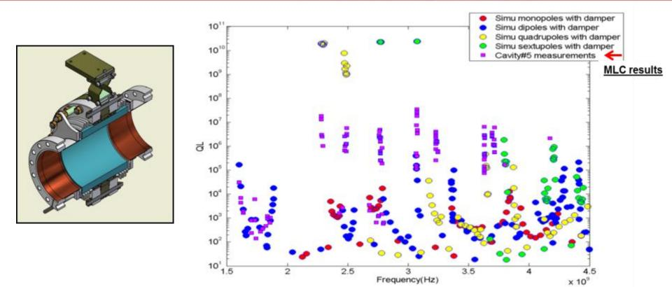
Dipole HOMs on IVILC were strongly damped below  $Q^{\sim}10^{\circ}$ . Consistent with HTC and simulation results.
