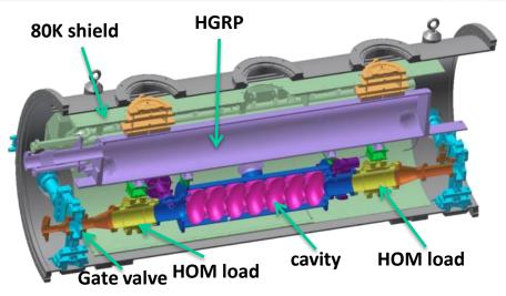
Horizontal Test Cryostat: 16MV/m, 1.8K: Q<sub>0</sub> = 2.E10 (reached with coupler)
