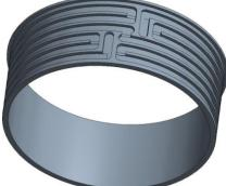
**Cooling Passage** Configuration of 80K **Cooling Jacket**
