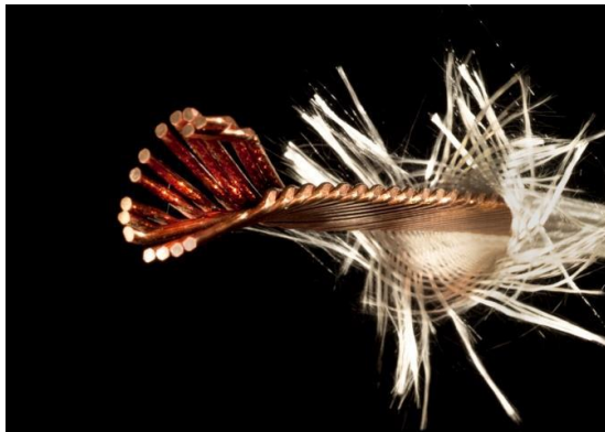
Development of Nb 3 Sn Conductor with J c almost 3 times of ITER
