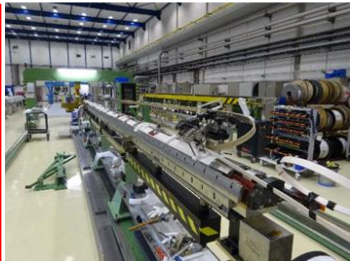
Insertion of coil package inside mechanical structure of the first IT quad prototypes (4.2 m long) in LBNL-USA
