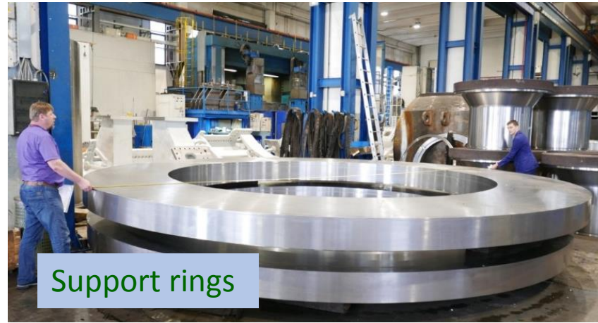
Aluminum support cylinder blanks for SC coil during transportation
