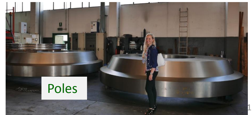
Aluminum support cylinder blanks for SC coil during transportation
