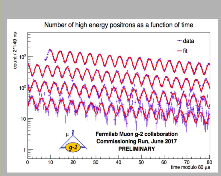
This figure was accumulated from two weeks of data accumulated in June 2017 and has approximately 700k positrons. The number of wiggles is somewhere between that achieved by CERN-II and CERN-III.
