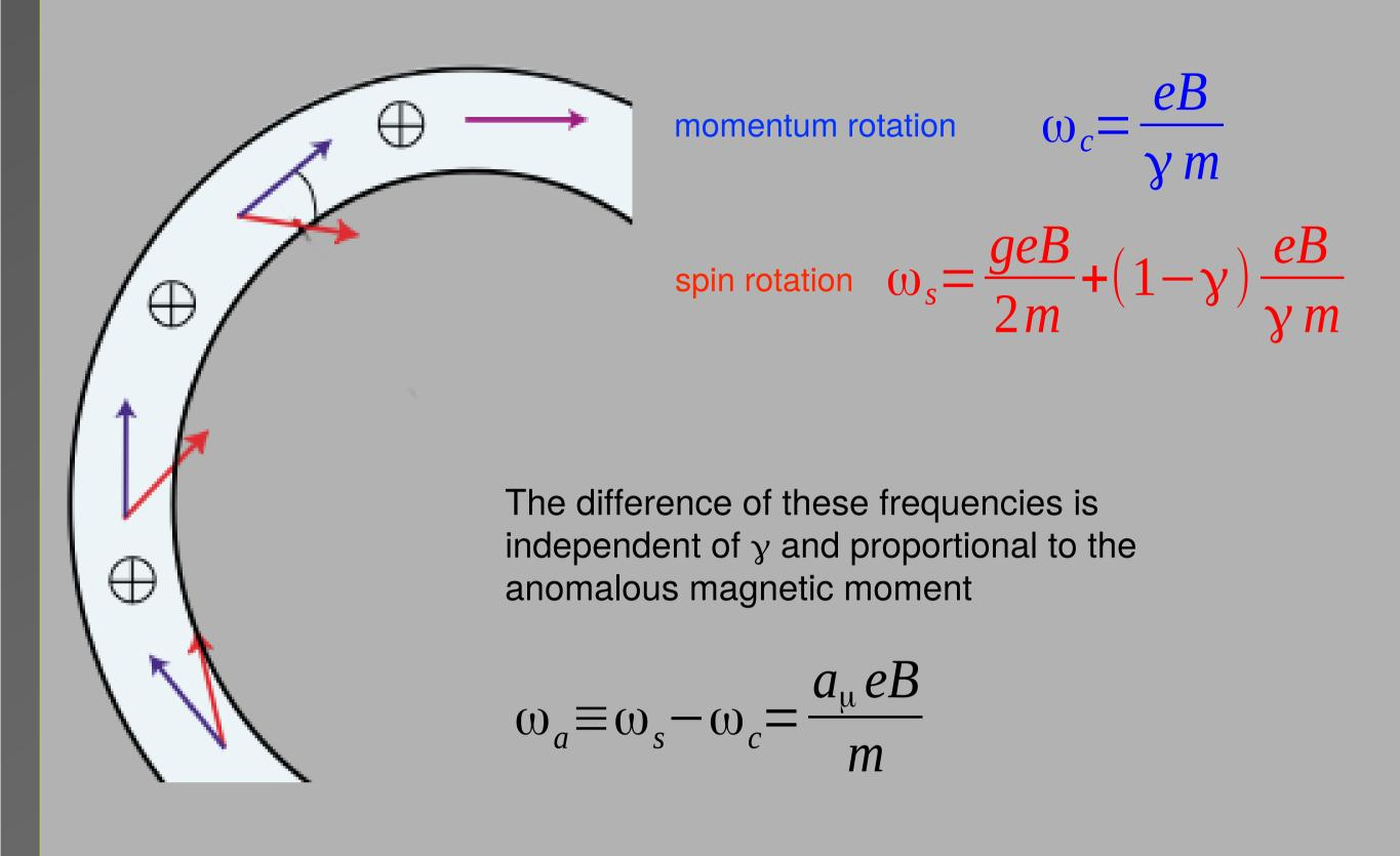
The quantity  $a_{\mu}$ , is obtained by measuring the frequency  $\omega_a$  and the magnetic field B, which can be absolutely tied to the precession frequency of free protons  $\omega_p$ .
