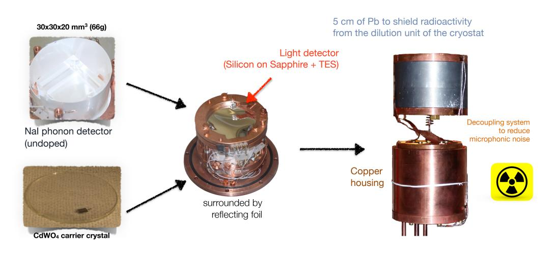
Construction and operation of first detector module for cryogenic operation
