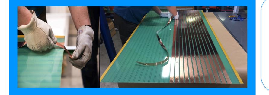
The MRPC signal pick-up electrodes are segmented into 24 strips, obtained by applying copper tape on vetronite panels. The strips are read out by NINO ASIC based front-end cards. The outer glass sheets are placed on the vetronite panels and a connection is made to the resistive coating, so that a high voltage can be applied.
