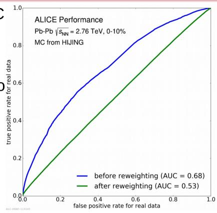
ROC curve of classifier: After reweighting, data and MC are hardly to separate in feature space
